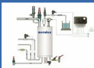
Automatic Air Purger for Refrigeration Plants
