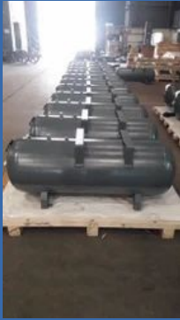
Air Receiver Tank
