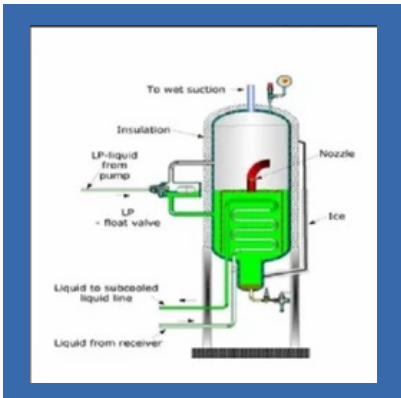
Water Refrigeration System Purger
